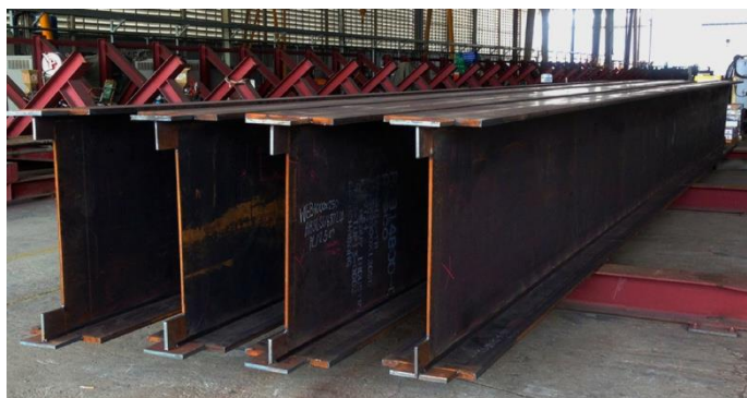
Fig.1 Built Beam – I Section with Plates connected on top and bottom flange
