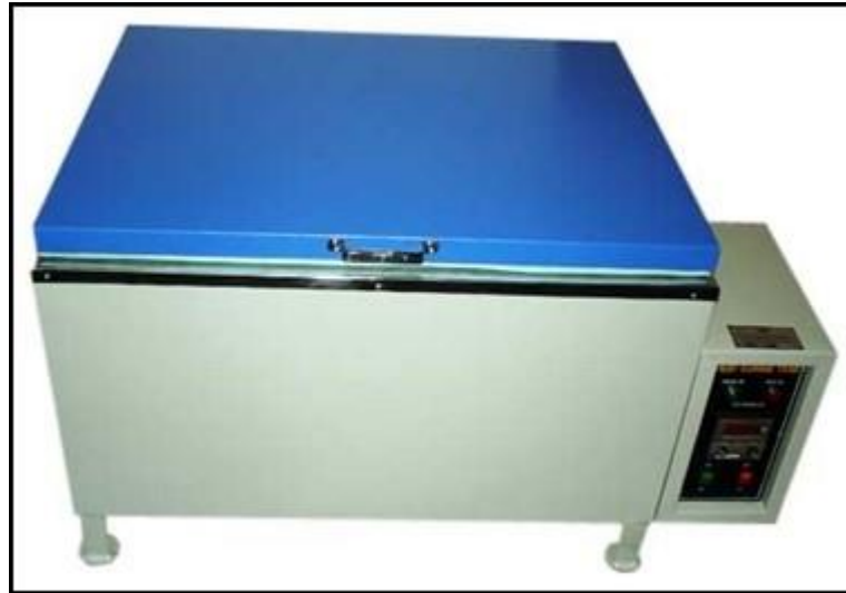
Accelerated curing tank used in laboratory for concrete testing
