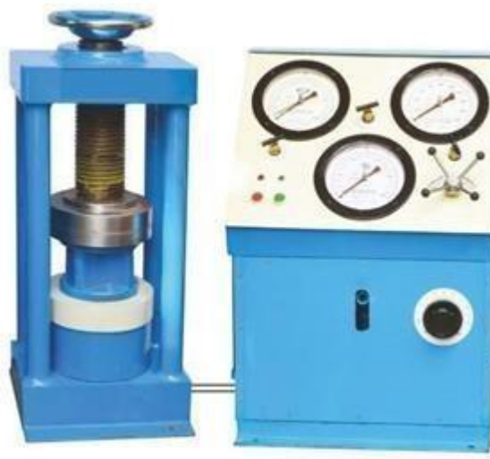
Compression test machine
