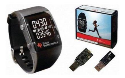
The <u>eZ430 Chronos</u> development kit from Texas Instruments represents great value for money and provides a wristwatch with a wireless-enabled microcontroller, accelerometers and temperature and barometric pressure sensors, and a USB programmer and RF access point. In this post I take a look at what it takes to get it up and running with a Raspberry Pi.
