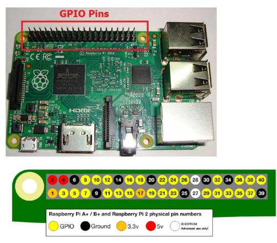
As shown in above figure, there are 40output pins for the PI. But when you look at the second figure, you can see not all 40 pin out can be programmed to our use. These are only 26 GPIO pins which can be programmed. These pins go from **GPIO2 to GPIO27**.
