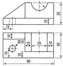
b) Draw the following views of the block shown pictorially. Use third-angle 5 M projection method. (i) Front view (ii) Top view (iii) side view
