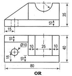
10 a) Draw the following views of the block shown pictorially in figure. Use 8 M third-angle projection method. (i) Front view (ii) Top view (iii) side view
