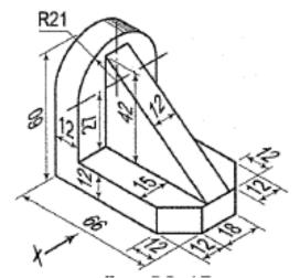
b) Draw the following views of the block shown pictorially in figure. Use 6 M third-angle projection method. (i) Front view (ii) Top view (iii) side view
