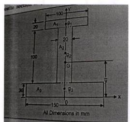
Find the coordinates of the centroid of the shaded area with respect to the axes as shown in fig,
