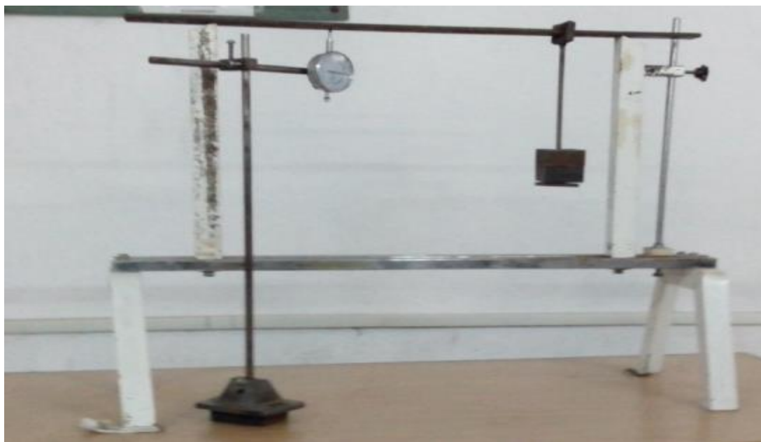
Simply supported Beam with Loads
