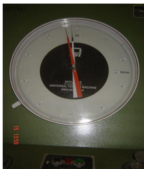
LOAD INDICATOR SYSTEM
