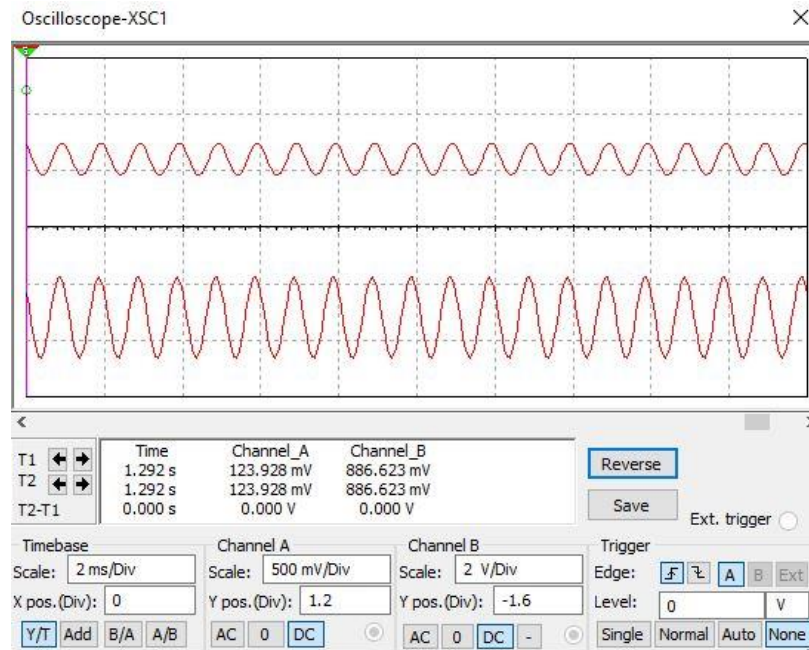
Fig: 2A.b Output waveform of cascade amplifier
