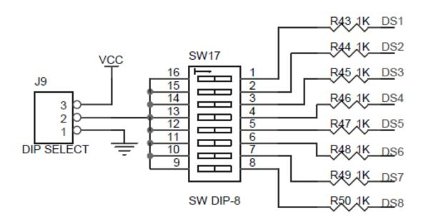
/\*------Example 1 : Read Switch status & displayed in LED's Description : Depends upon the dip switch position the corresponding leds are on (or) off ------\*/
